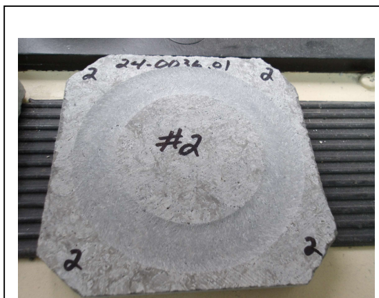
Photo No. 20 ASTM C1353 – Representative Post-Abrasion Specimen Condition
