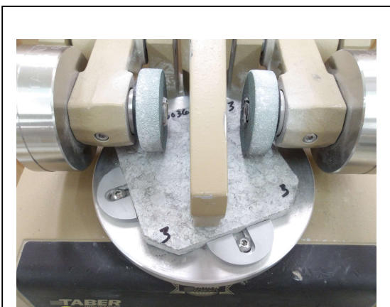
Photo No. 19 ASTM C1353 – Test in Progress
