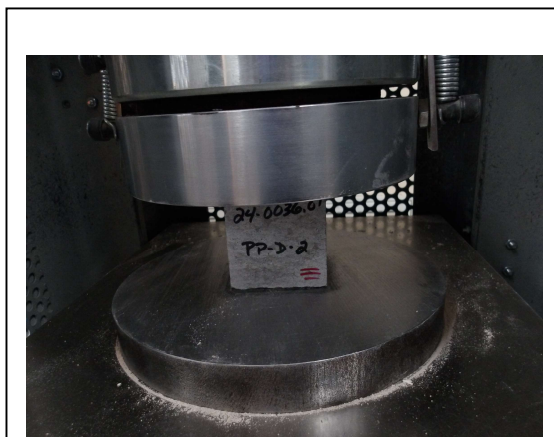
Photo No. 2 ASTM C170 – Test Setup
