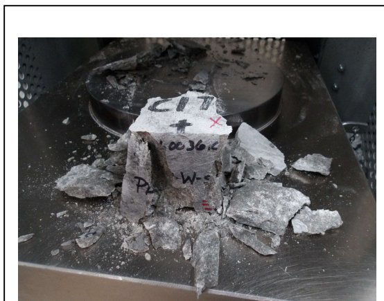
Photo No. 4 ASTM C170 – Specimen Failure Mode: Loading Perpendicular to Rift (Wet Condition)
