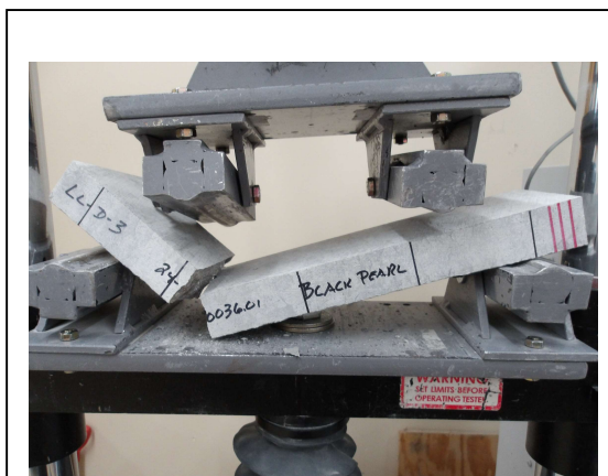
Photo No. 12 ASTM C880 – Specimen Failure Mode: Loading Parallel to Rift (Dry Condition)
