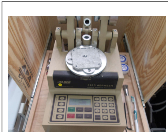
Photo No. 18 ASTM C1353 – Abrasion Test Setup
