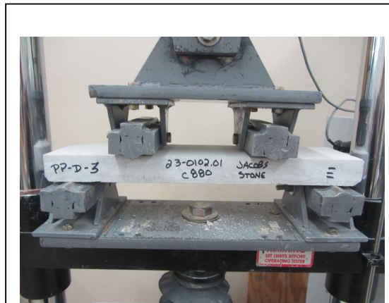
Photo No. 10 ASTM C880 – Specimen Loading Detail
