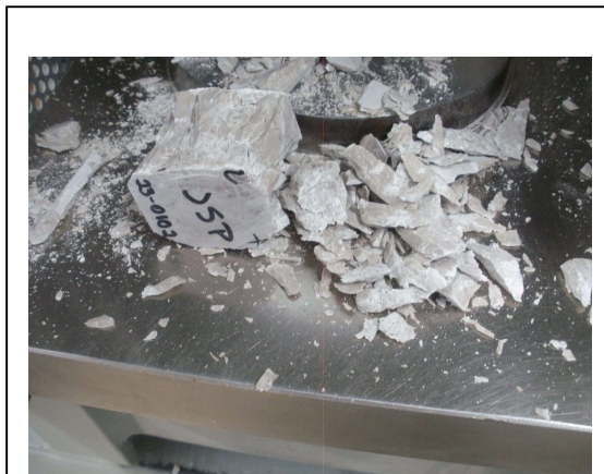
Photo No. 4 ASTM C170 – Specimen Failure Mode: Loading Parallel to Rift (Dry Condition)
