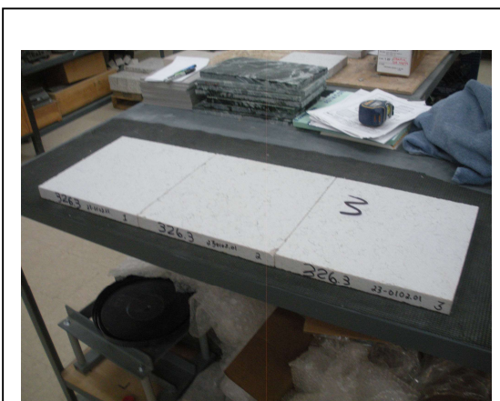
Photo No. 24 DCoF Test Set Up
