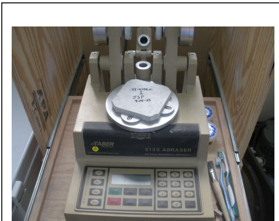
Photo No. 18 ASTM C1353 – Abrasion Test Setup
