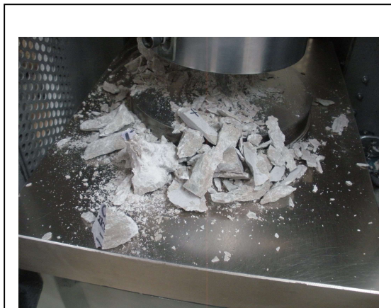
Photo No. 3 ASTM C170 – Specimen Failure Mode: Loading Perpendicular to Rift (Wet Condition)
