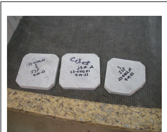
Photo No. 17 ASTM C1353 – Pretest Specimen Condition
