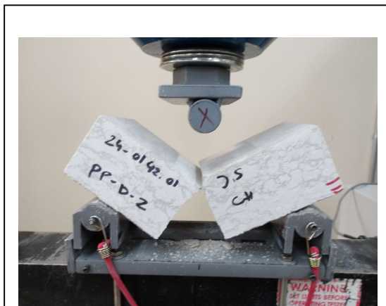
Photo No. 7 ASTM C99 – Specimen Failure Mode: Loading Perpendicular to Rift (Dry Condition)
