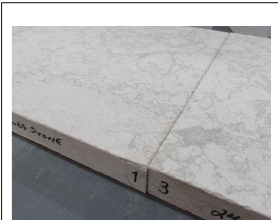
Photo No. 23 Surface Detail – Chapel Hill Limestone (Sawn Finish)
