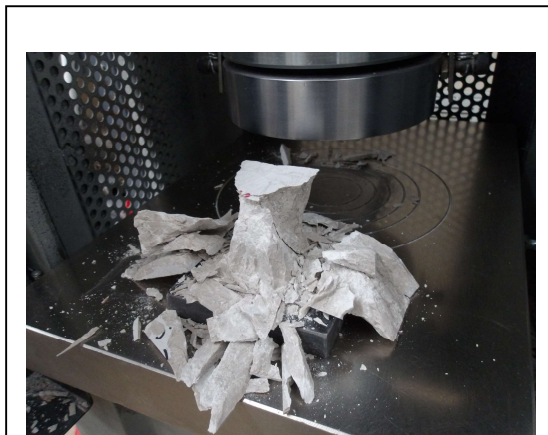
Photo No. 3 ASTM C170 – Specimen Failure Mode: Loading Parallel to Rift (Dry Condition)
