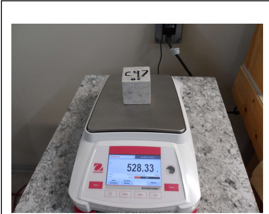
Photo No. 9 ASTM C97 – Absorption & Density Specimen Test Setup
