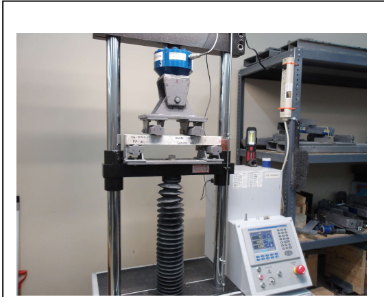
Photo No. 10 ASTM C880 – Flexural Strength Test Setup
