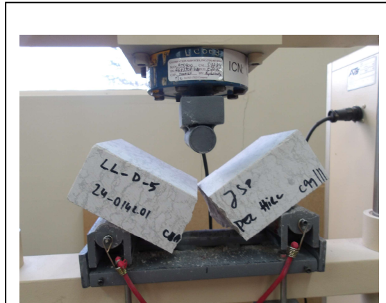
Photo No. 6 ASTM C99 – Specimen Failure Mode: Loading Parallel to Rift (Dry Condition)
