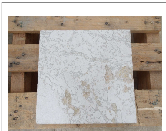
Photo No. 27 ASTM C1645 – Specimen No. 3 Underside Facing (Maximum Rear Face Spalling Specimen Condition Observed)
