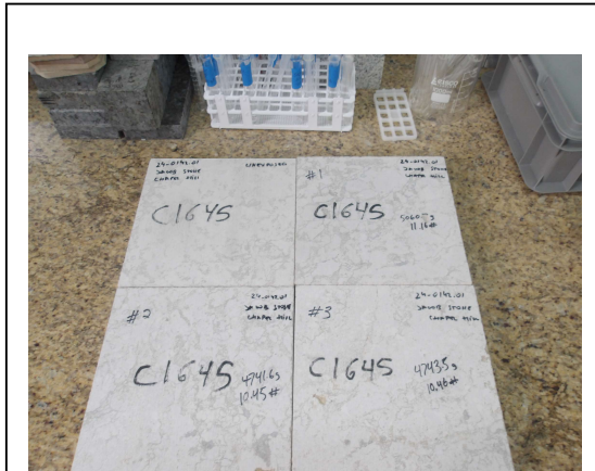
Photo No. 25 ASTM C1645 – Comparative Post-Exposure Exterior Facing (Unexposed Control Depicted Top Left, Post-Exposure Depicted Top Right, Bottom Left and Right)
