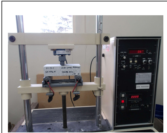
Photo No. 5 ASTM C99 – Modulus of Rupture Test Setup
