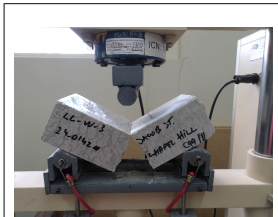
Photo No. 8 ASTM C99 – Specimen Failure Mode: Loading Parallel to Rift (Wet Condition)
