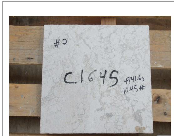
Photo No. 26 ASTM C1645 – Specimen No. 2 Exterior Facing (Maximum Top Face Spalling Specimen Condition Observed)
