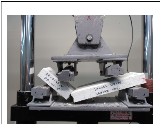
Photo No. 12 ASTM C880 – Specimen Failure Mode: Loading Parallel to Rift (Wet Condition)
