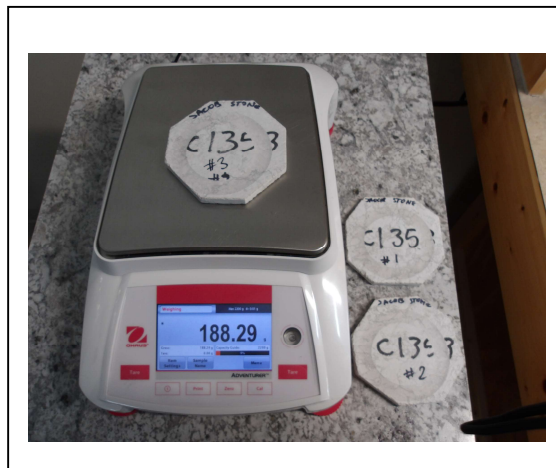
Photo No. 20 ASTM C1353 – Post-Abrasion Specimen Condition
