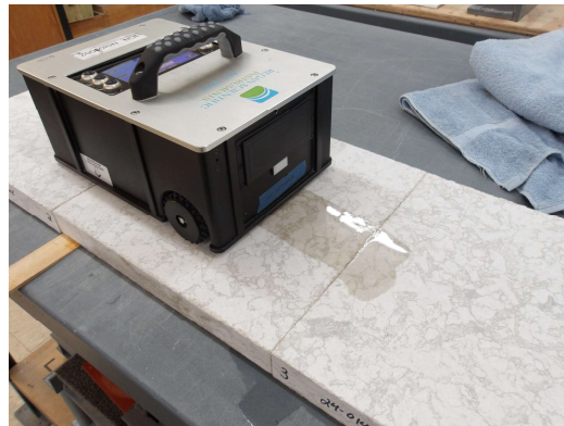
Photo No. 24 ANSI A326.3 – DCOF Test in Progress
