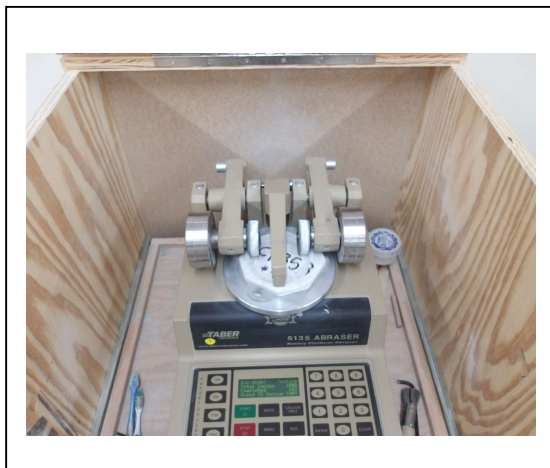
Photo No. 19 ASTM C1353 – Test in Progress
