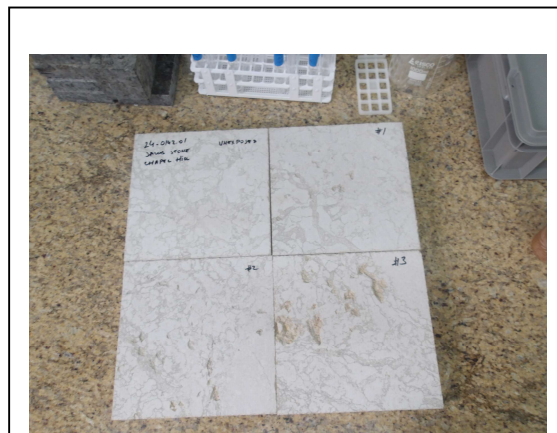
Photo No. 28 ASTM C1645 – Comparative Post-Exposure Underside Facing (Unexposed Control Depicted Top Left, Post-Exposure Depicted Top Right, Bottom Left and Right)
