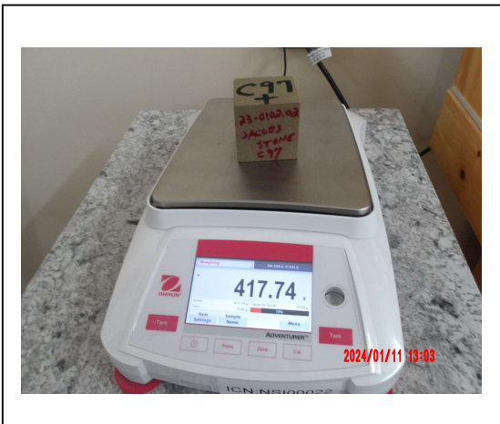
Photo No. 5 ASTM C97 – Absorption & Density Test Setup (Wet Mass Determination Depicted)
