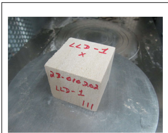
Photo No. 1 ASTM C170 – Representative Pretest Condition Specimen
