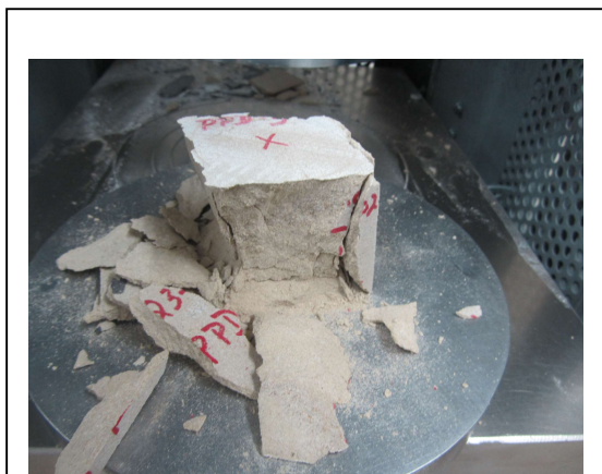
Photo No. 3 ASTM C170 – Specimen Failure Mode: Loading Perpendicular to Rift (Dry Condition)
