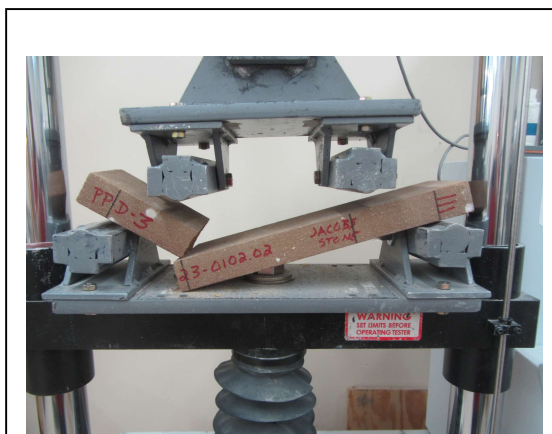
Photo No. 12 ASTM C880 – Specimen Failure Mode: Loading Perpendicular to Rift (Wet Condition)
