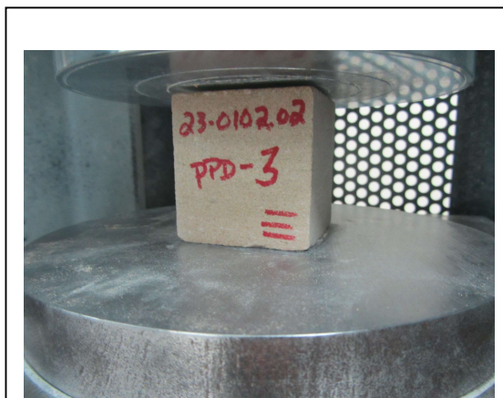
Photo No. 2 ASTM C170 – Test Setup
