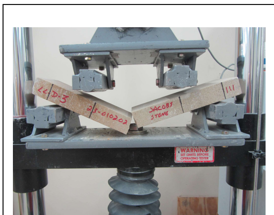
Photo No. 11 ASTM C880 – Specimen Failure Mode: Loading Parallel to Rift (Dry Condition)
