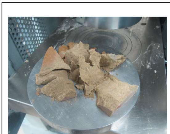
Photo No. 4 ASTM C170 – Specimen Failure Mode: Loading Parallel to Rift (Wet Condition)
