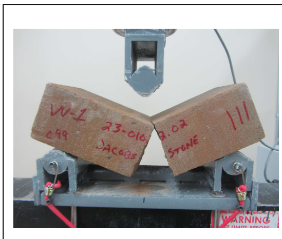
Photo No. 8 ASTM C99 – Specimen Failure Mode: Loading Parallel to Rift (Wet Condition)
